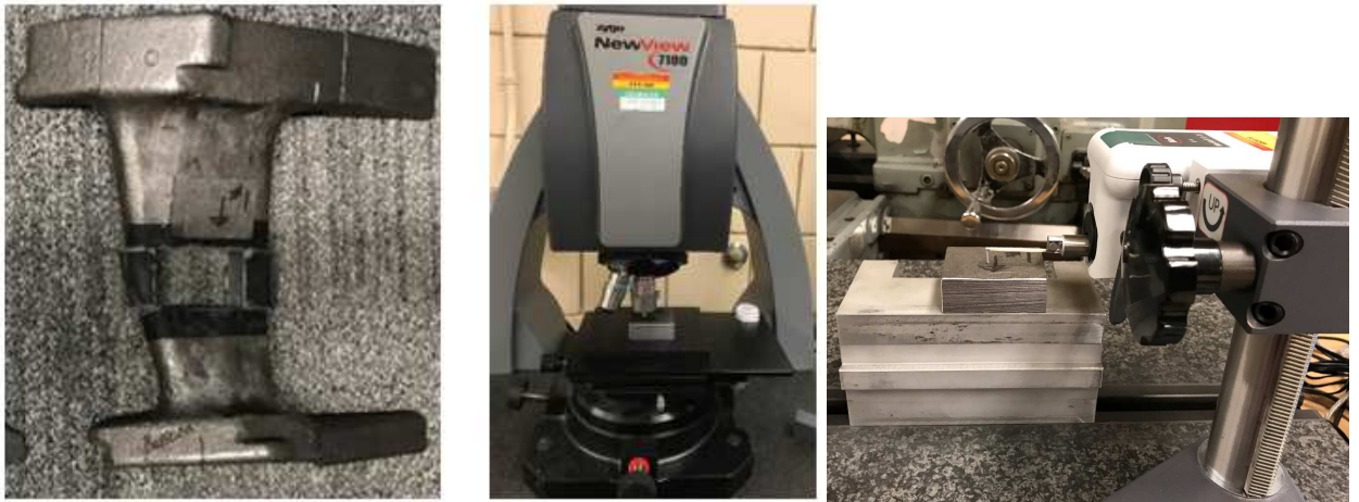
Figure 41: Cut sample from Casting C and sample measurement using Zygo surface profiler and Mahr profilometer.
