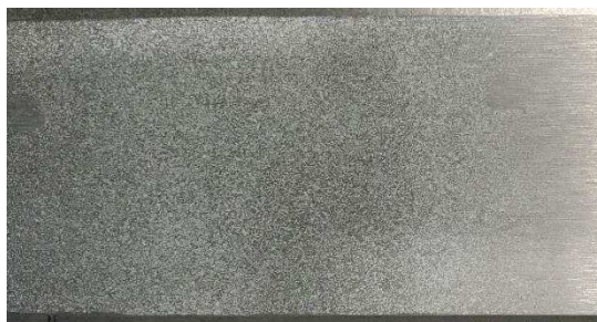
Figure 18: Surface of a precision machined flat plate coated with dulling spray
