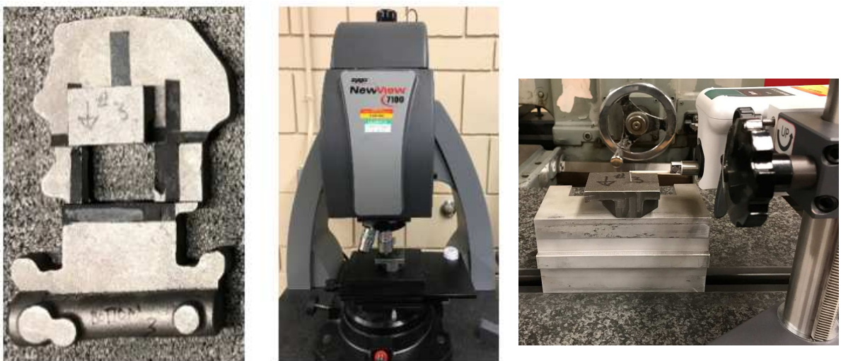
Figure 35 : Cut samples from Casting A-1 and sample measurement on Zygo surface profiler and Mahr profilometer.
