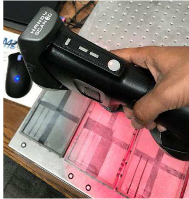
Figure 42: HandyScan700 capturing point cloud of SCRATA plates
