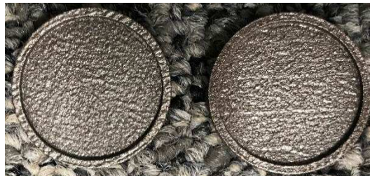
Figure 45: SS316L sample as fabricated by DMLS process
