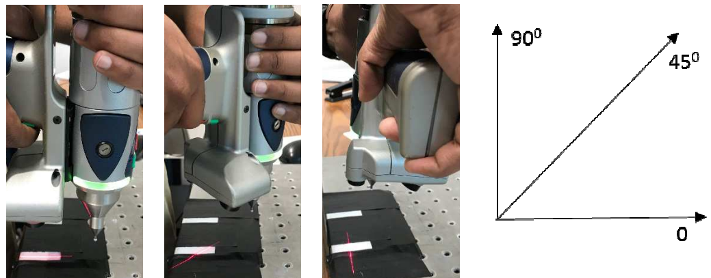
Figure 21: Laser scanning setup showing 0, 45 and 90 degree scanning direction along with a graphical schematic
