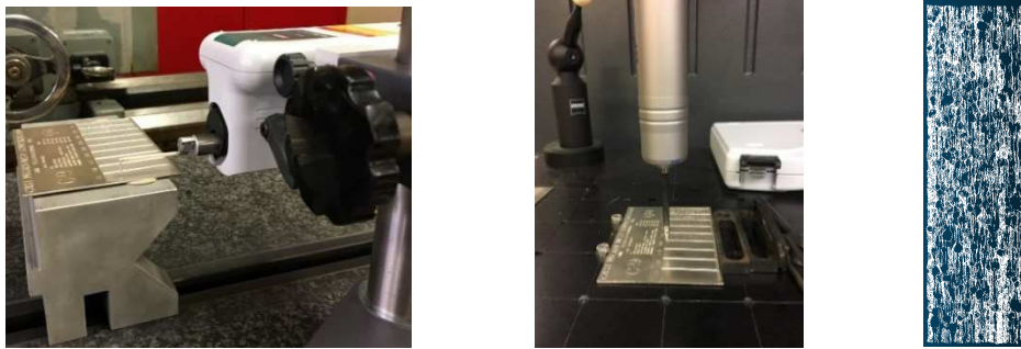
Figure 5: a) Mahr SD 26 Profilometer, b) Zeiss CMM and c) 720 \mu\text{m} point cloud generated by the CMM
