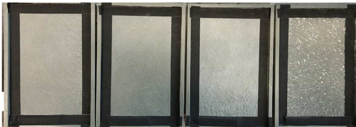
Figure 29: ASTM A802 – SCRATA Surface Texture Plates (left to right- A1 to A4)
