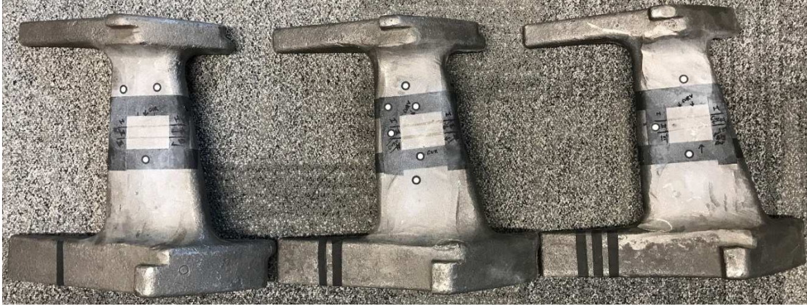
Figure 39: Sections of three Casting C within black masking tape representing areas of scanning on three identical surfaces
