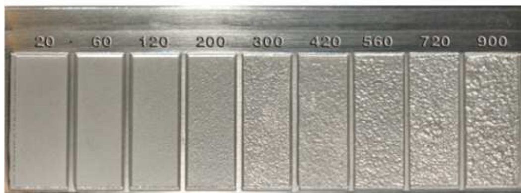
Figure 15: ‘C-9’ Micro finish Comparator with varying surface finishes from 20 to 900 RMS
